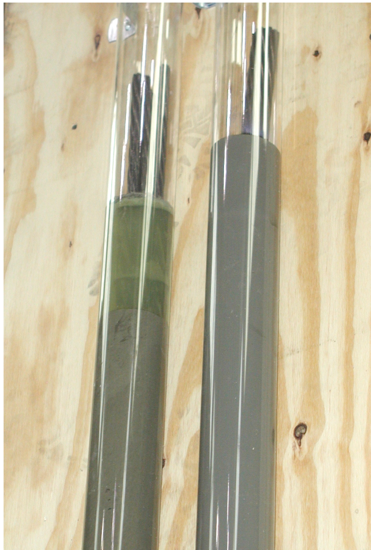
Figure 3.12 Closer View of Vertically Grouted Tendons 36
