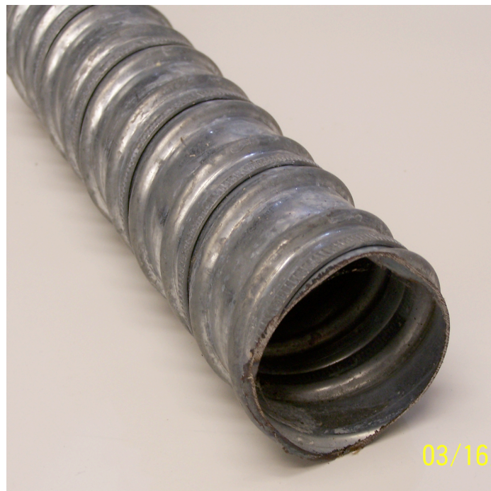
Figure 3.6 Corrugated Galvanized Steel Duct 25
